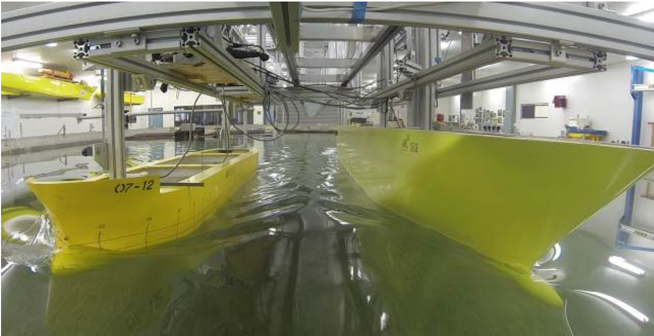
Figure 6 Photograph of RAS experiments to investigate the influence that both lateral and longitudinal separations between vessels have on the interactions. It was found that this can lead to large supply vessel (left) roll motions in head seas and that variations in lateral and longitudinal separation between vessels had a large influence on the peak roll response of the supply vessel [20].
