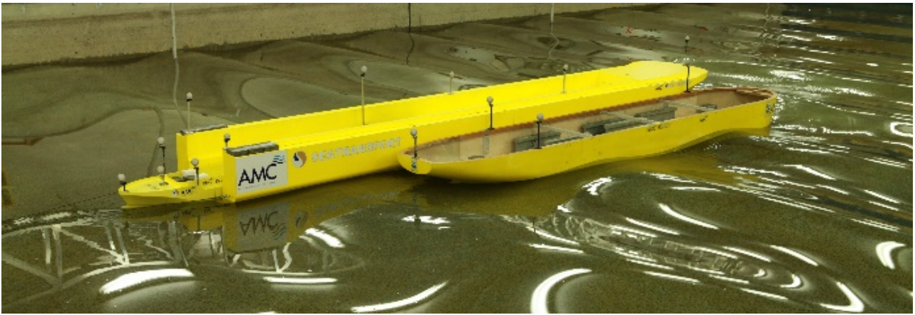
Figure 9 A photograph from recent experiments involving the 5m long scale model of the FHT, feeder vessel and ocean going vessel in the AMC shallow water wave basin. The bow of the feeder vessel can be seen protruding from the FHT well dock (left). Both Panamax and Capesize ocean going vessels are under consideration: the smaller Panamax size is shown here. A minimum of four markers (silver spheres) are fixed to each of the three models to allow the Qualisys optical motion tracking system to measure all six degrees of motion for each ship model. The incident waves seen here are regular head seas, but the study is investigating a number of irregular wave spectra and wave headings.
