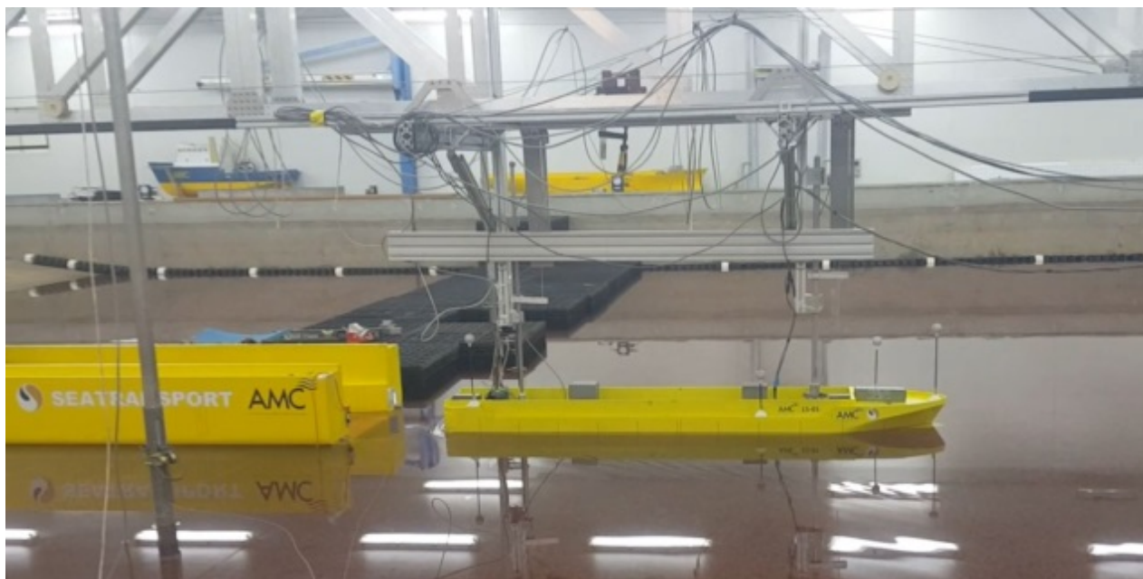
Figure 5 Photograph showing the scale model of the feeder vessel (right) about to travel astern to enter the stern well dock in the model of the FHT (left). In addition to acquiring PIV data of the complex flow inside the well dock as the feeder performs this manoeuvre, the dynamic effects on the hull resistance (powering requirements) and motions were also quantified.
