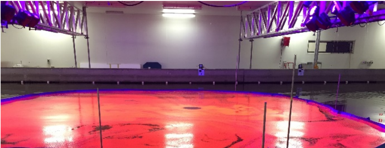
Figure 1 A photograph of the experimental set-up for the stereo videogrammetry. The cameras and UV lights are mounted on the raised trusses and the surging active WEC model lies submerged beneath the pink fluorescing particles floating on the water surface.
