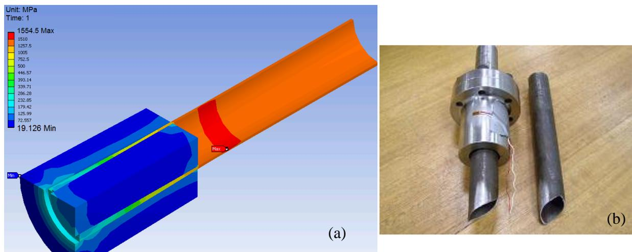
Figure 2. Comparison of the stress in the model (a) with the failure in the test sample (b) (Jiao et al. 2011)
