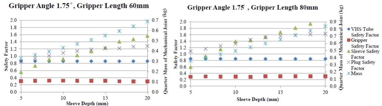
Figure 3. Safety factor versus the sleeve depth
