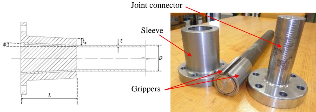
Figure 1. Mechanical joint configuration (Jiao et al. 2011)
