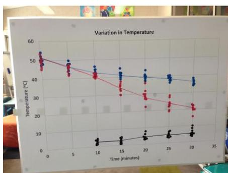
Figure 3. Graph showing the results of the heat experiment for all the groups, showing variation among conditions (top line: insulated cup, middle: plain cup; bottom: ice water), over time, and across groups (dots).
