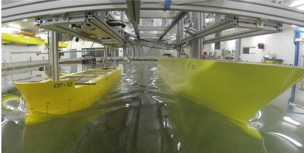
Figure 6 Photograph of RAS experiments to investigate the influence that both lateral and longitudinal separations between vessels have on the interactions. It was found that this can lead to large supply vessel (left) roll motions in head seas and that variations in lateral and longitudinal separation between vessels had a large influence on the peak roll response of the supply vessel [20].
