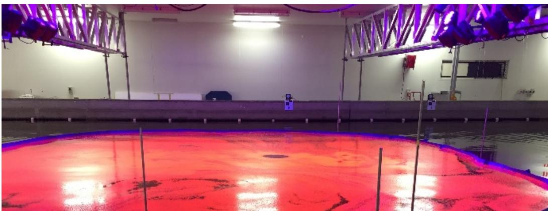
**Figure 1** A photograph of stereo videogrammetry experimental set-up. The cameras and UV lights are mounted on the raised trusses and the surging active WEC model lies submerged beneath the pink fluorescing particles floating on the water surface.
