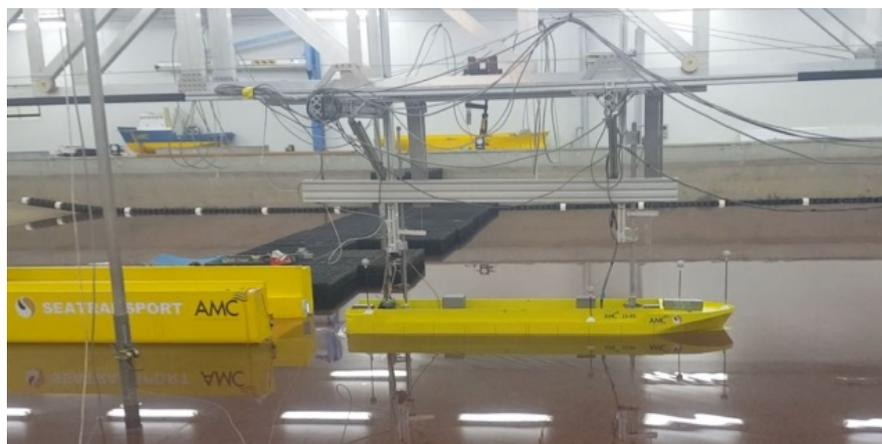
**Figure 5** Photograph showing the scale model of the feeder vessel (right) about to travel astern to enter the stern well dock of the FHT (left). In addition to acquiring PIV data of the complex flow inside the well dock as the feeder performs this manoeuvre, the dynamic effects on the hull resistance (powering) and motions were also quantified.
