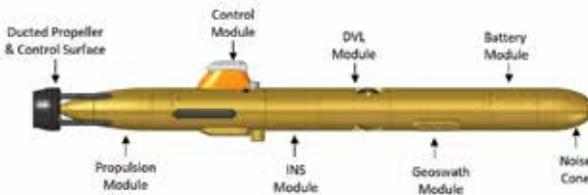
Figure 4: The configuration of the utilized *Gavia* class AUV consisted of a nose cone, battery module, Geoswath module, DVL module, INS module, Control module, Propulsion module, and ducted propeller and control surfaces.
