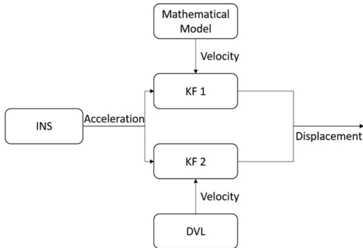
Figure 1: The block diagram of an overall process for model-aided INS localization. Once INS measures acceleration data from AUVs' trials, the data are combined and amended with a mathematical model using KF (MA-INS). INS data are also combined with DVL result by another KF, and the data are applied to MA-INS intermittently.
