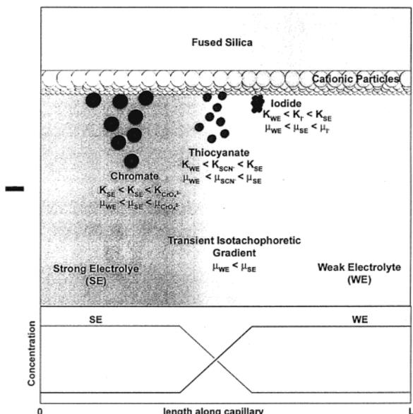
Figure 2. Schematic representation of the focusing mechanism using an IE-OT-CEC column and a transient-isotachophoretic gradient, illustrated by  $I^-$ .  $SCN^-$  is not focused because its electrophoretic mobility is lower than that of the SE, while  $CrO_4^{2-}$  is not focused because the eluotropic strength of the SE is too low.
