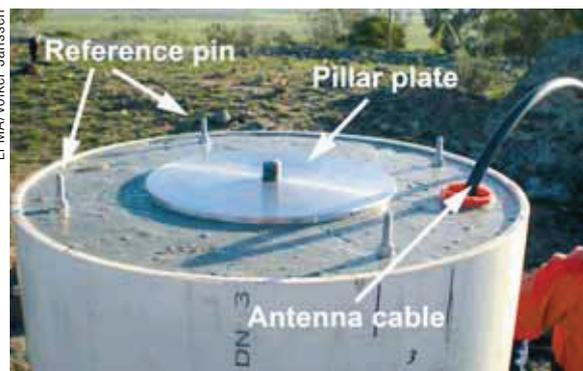
Pillar plate with reference pins (top) and symmetrically coupled points on the antenna used in the indirect survey (bottom)
