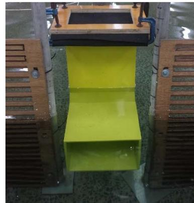
Fig. 4. OWC model integrated in the porous breakwater with no solid fitting.
