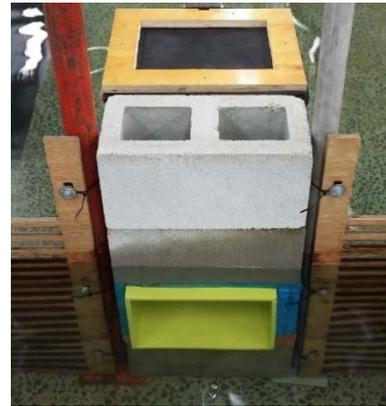
Fig. 3. Solid wall fitting simulation for model scale OWC device integrated within porous breakwater.
