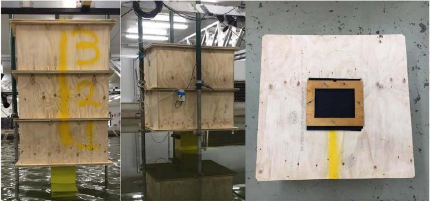
Fig. 3 Model scale OWC device fitted with additional 1.5 m<sup>3</sup> air chamber (left), 1 m<sup>3</sup> air chamber (middle) and PTO simulant secured using sealing plate (right)
