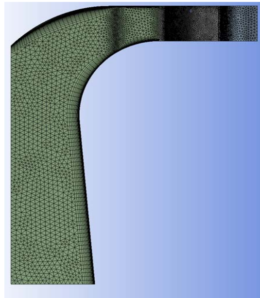
Fig. 5 schematic of the mesh used in the duct section in the numerical simulations..
