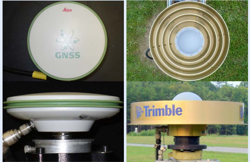
Figure 2: Different antenna designs: (left) a typical rover antenna (LEIAX1203+GNSS), and (right) a typical choke ring antenna (TRM59800.00), often used for CORS (US National Geodetic Survey).
