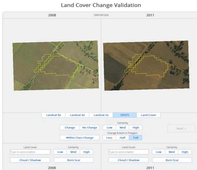
**Figure 4. Web-based land cover change detection validation interface using SPOT5 2.5m pan-sharpened merged product.**
