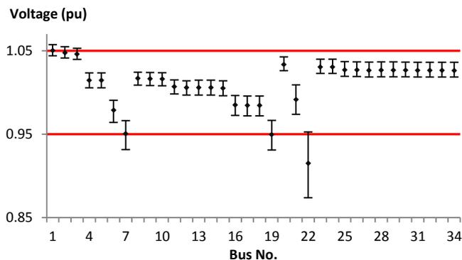
Fig. 4. The 95% confidence interval for the base loading condition without distributed generation (Case 1).
