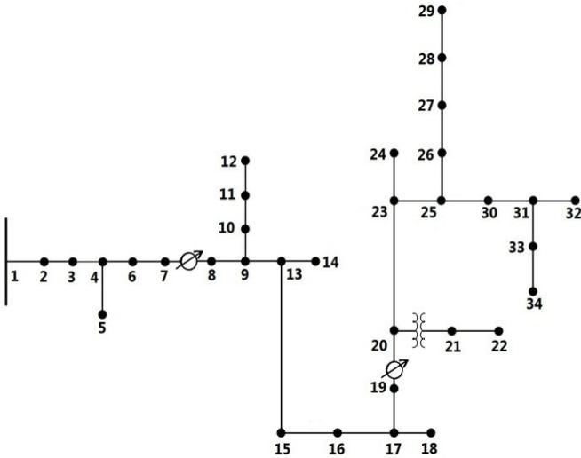
Fig. 1. The 34-bus test feeder.
