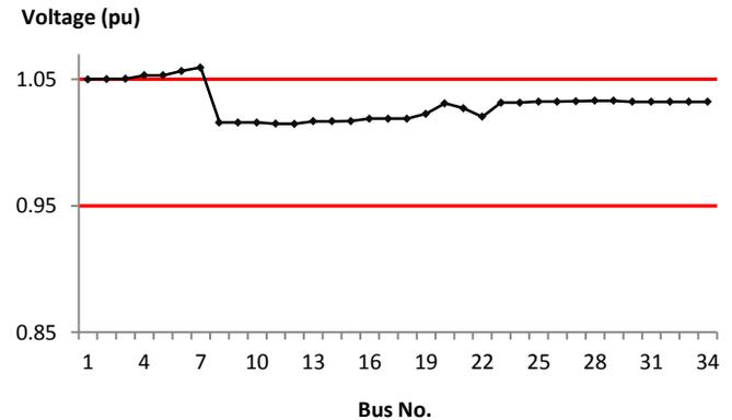
Fig. 3. The voltage profile for the 34-bus test feeder under low loading condition with distributed generation (Case 2).
