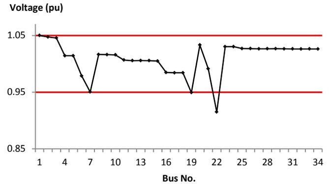
Fig. 2 The voltage profile for the 34-bus test feeder under base loading condition without distributed generation (Case 1).
