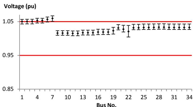
Fig. 5. The 95% confidence interval for the low loading condition with distributed generation (Case 2).
