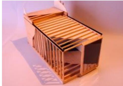
Figure 3: Cut-away scale model of a module. Images credit: Morrison & Breytenbach Architects
