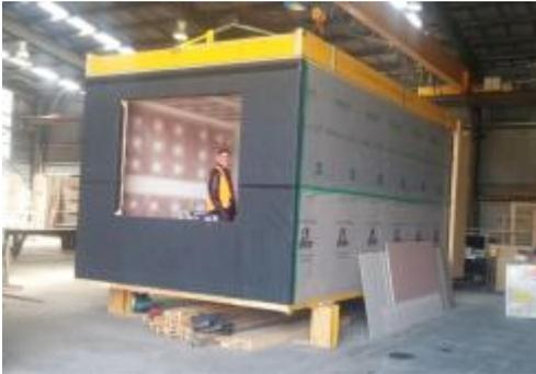
Figure 6: Wrapped and lined prototype with test floor over.
