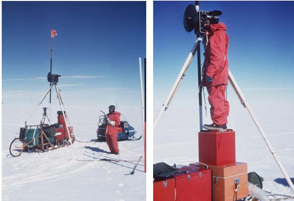
Fig. 3: Tellurometer set-up at a 'Corry' pole in 1970. The sledge-wheel is visible on the left. Photographs by Max Corry (left) and Norman Linton-Smith (right), Australian Government Antarctic Division © Commonwealth of Australia.
