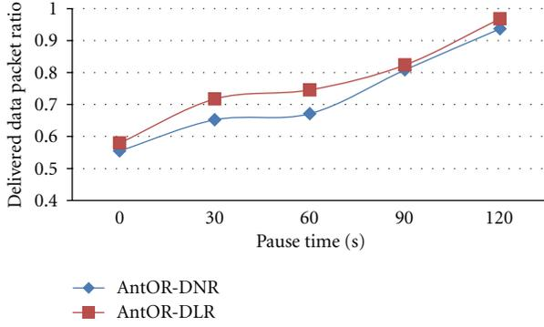
FIGURE 1: Pause time against delivered data packet ratio.
