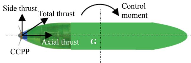
Fig. 3 Conceptual axial and side thrusts of a CCPP for steering a ROV/AUV in all directions.
