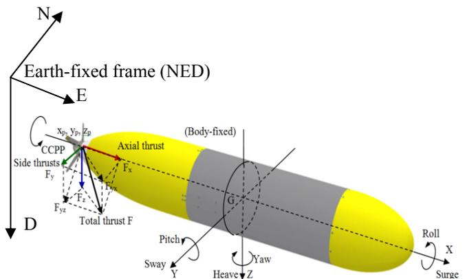
Fig. 8 Reference frames and the ROV/AUV with a CCPP.
