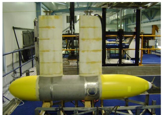
Fig. 5 ROV/AUV with CCPP and force and moment balance mechanism.
