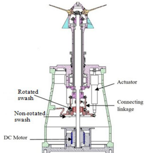
Fig. 4 Cross section drawing of the CCPP
