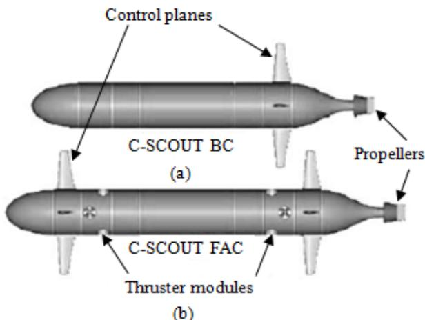
Fig. 1 A typical conventional propulsion system for a streamlined ROV/AUV (Perrault, 2002 and Evans, 2003).
