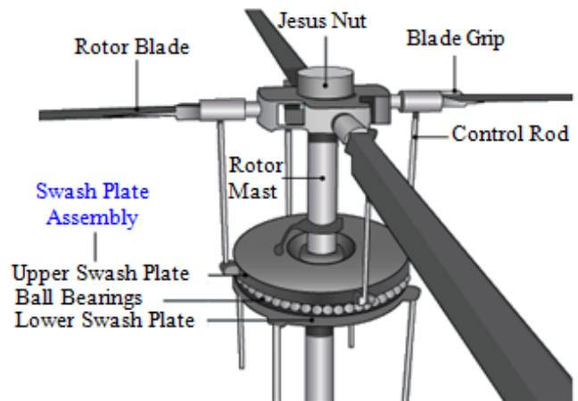
Fig. 2 A helicopter propeller with four blades and rotor (Brain and Harris, 2013).
