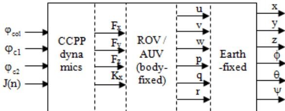
Fig. 9 Inputs and outputs of the ROV/AUV with CCPP.
