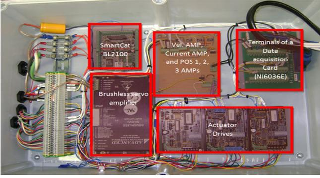
Fig. 10 Control electronics for the CCPP.
