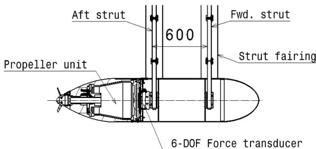
Fig. 7 Set-up configuration in a cross section view.
