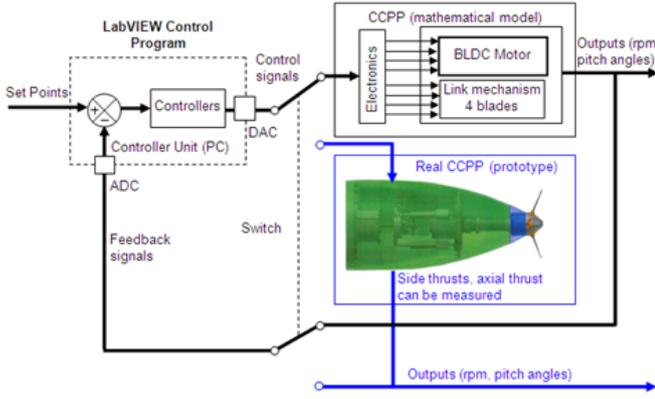
Fig. 11 Functional block diagram of the CCPP.
