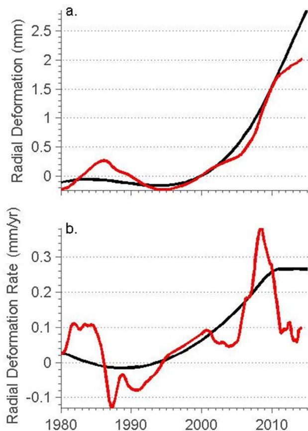
**Figure 3.** (a) Radial deformation at maxima; (b) radial deformation rate at the maxima. Deformation patterns at the minima are identical but of opposite sign. The black lines are computed using the IERS 2010 model, the red lines using our filtered C04 time-series.
