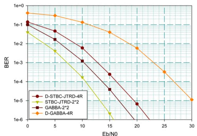
Fig. 2 BER of GABBA and STBC-JTRD (P2P and distributed AF network)
