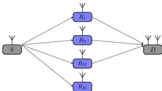
Fig. 1 AF relaying network model
