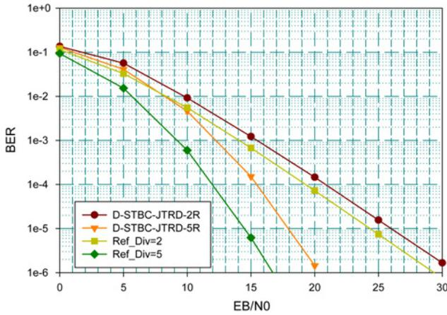
Fig. 3 BER of  $1 \times 2 \times 2$  and  $1 \times 5 \times 2$  D-STBC-JTRD scheme
