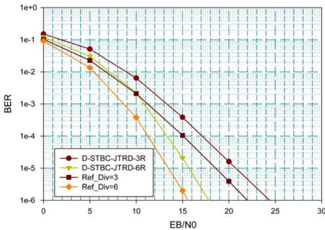
Fig. 4 BER of  $1 \times 3 \times 2$  and  $1 \times 6 \times 2$  D-STBC-JTRD scheme
