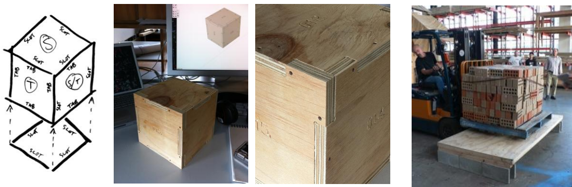
Figure 3. Translation of drawing into digital model into physical object and panel testing
