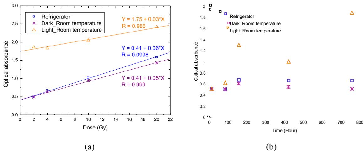
**Figure 3:** The optical absorbance of irradiated PRESAGE<sup>®</sup> cuvettes (a) versus dose, at 633 nm, 80 hours after the irradiation and (b) for 20 Gy dose, at 670 nm, over a period of post-irradiation time in the fridge, in the dark at room temperature and in the light at room temperature.
