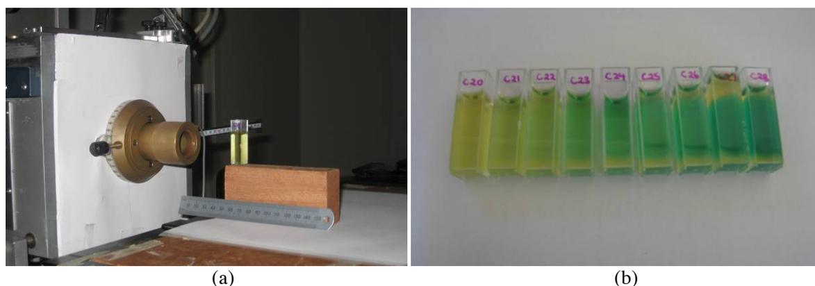
**Figure 1:** (a) Placement of PRESAGE<sup>®</sup> cuvettes in front of an unmodulated 62 MeV proton beam and (b) irradiated PRESAGE<sup>®</sup> cuvettes with a dose range of 0.5 Gy – 8 Gy.
