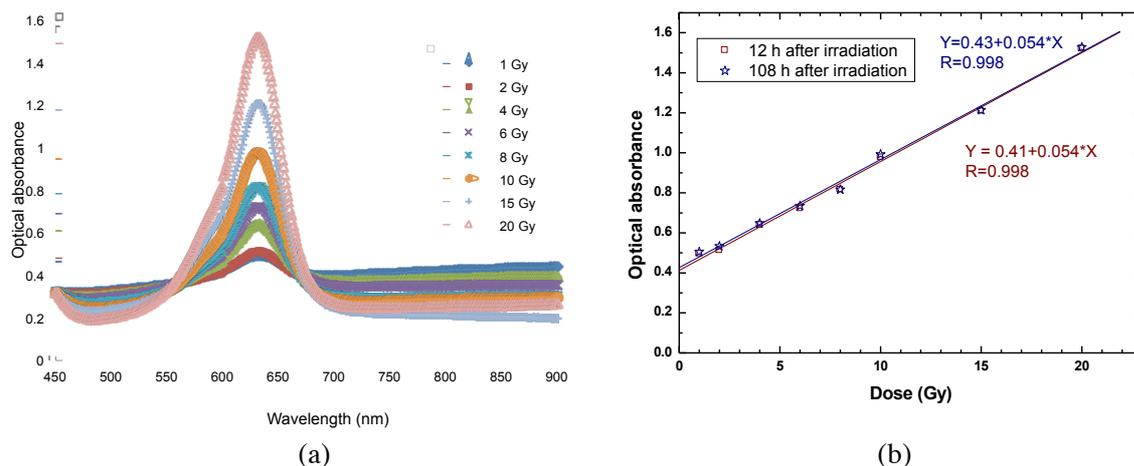
**Figure 2:** The optical absorbance of nine irradiated PRESAGE<sup>®</sup> cuvettes by an unmodulated 62 MeV proton beam (a) 12 hours after irradiation and (b) at 633 nm 12 hours and 108 hours after irradiation by.
