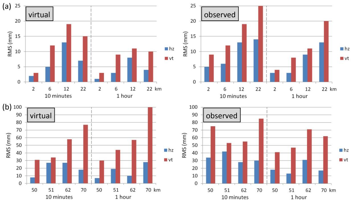
**Figure 6:** Comparison of virtual and observed baseline results against the ‘true’ position for two observation windows and different baseline lengths in the horizontal (hz) and vertical (vt) components for (a) Queens Square (small cell) and (b) Sofala (large cell).
