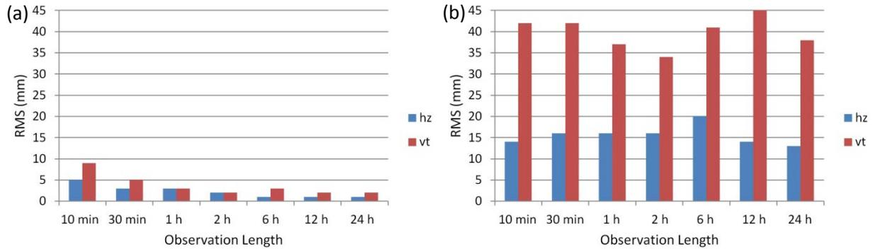
**Figure 3:** ‘Zero’ baseline results in the horizontal (hz) and vertical (vt) components for (a) Queens Square (small cell) and (b) Sofala (large cell).
