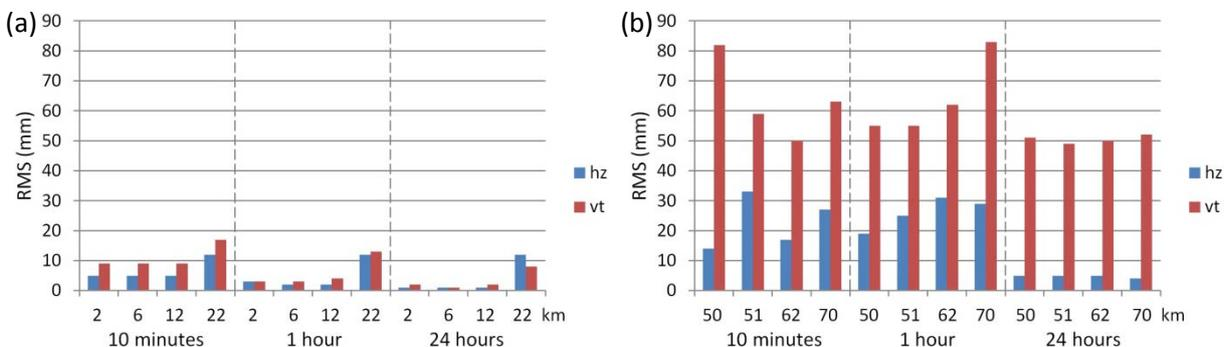
**Figure 5:** Baseline results for increasing observation windows and different baseline lengths in the horizontal (hz) and vertical (vt) components for (a) Queens Square (small cell) and (b) Sofala (large cell).
