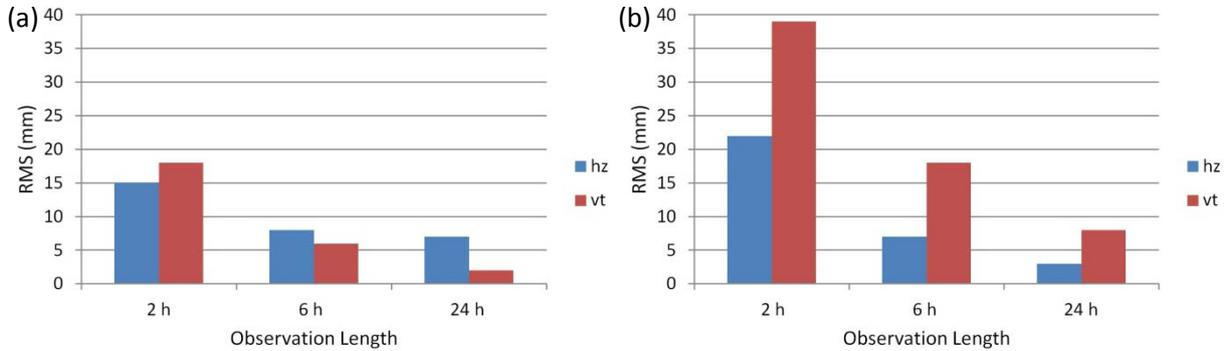
**Figure 4:** AUSPOS results in the horizontal (hz) and vertical (vt) components for (a) Queens Square (small cell) and (b) Sofala (large cell).
