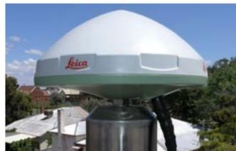
Figure 3: Antenna monument with bevelled edge.
