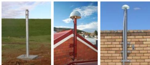
Figure 2: CORSnet-NSW free-standing pole and wall monuments.
