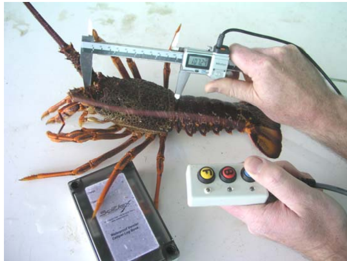
Figure 4. Measuring a lobster using an electronic data logger.
