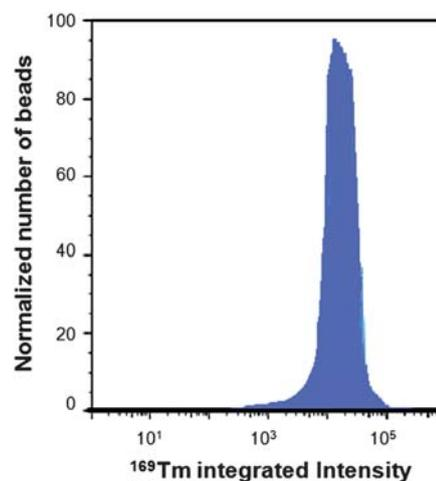
**Fig. 3** Distribution of mass cytometry intensity signal for a population of PS beads (AA086-Tm) prepared by 2-DisP in presence of  $\text{TmCl}_3$  (0.1 wt%/styrene) and AA (2.0 wt%/styrene).
