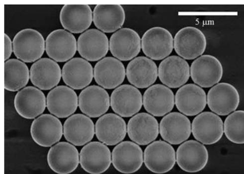
**Fig. 1** SEM image of PS bead sample AA070-Tm synthesized in the presence of 1% TmCl<sub>3</sub> added in the second stage with AA: 2 wt %/styrene ( $d = 2.1 \mu\text{m}$ ,  $CV_d = 2.5\%$ ).
