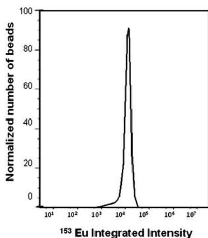
**Fig. 5** Distribution of mass cytometry signal intensity for a population of PS beads (AA120-Eu) prepared by 3-DisP in presence of  $\text{EuCl}_3$  (0.1 wt%/styrene) and AA (4.0 wt%/styrene).  $\text{CV}_{\text{Eu}} = 14\%$ .
