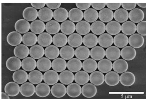
**Fig. 4** SEM image of PS bead sample AA120-Eu synthesized by 3-DisP in the presence of 0.1%  $\text{EuCl}_3$  added in the second stage with AA: 4 wt %/styrene ( $d = 2.2 \mu\text{m}$ ,  $\text{CV}_d = 1.6\%$ ).
