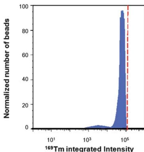
**Fig. 2** Distribution of mass cytometry intensity signal for a population of PS beads (AA070-Tm) prepared by 2-DisP in presence of  $\text{TmCl}_3$  (1.0 wt%/styrene) and AA (2.0 wt%/styrene). The dashed-line indicates the sharp cutoff at *ca.*  $10^5$   $^{169}\text{Tm}$  signal intensity that this is likely due to detector saturation.
