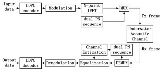
**Figure 4. TDS-OFDM system for underwater acoustic channel.**
