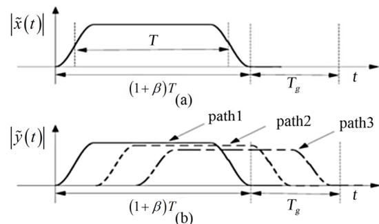
**Figure 3. Illustration of the transmitted and received signals in the time domain. (a) One transmitted ZP-OFDM block; (b) One received ZP-OFDM block.**
