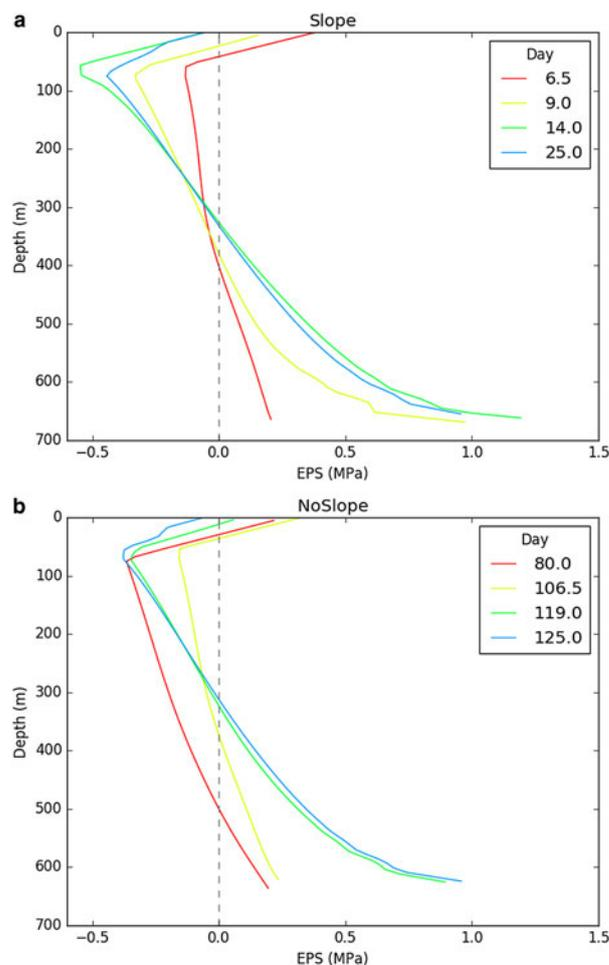
**Fig. 9.** Vertical transects of effective principal stress above the ungrounding point for selected time steps in (a) the sloping bed case; (b) the horizontal bed case. Calving occurred in HiDEM for the ice geometries at 14 and 25 days (sloping bed) and 119 and 125 days (horizontal bed), but not at the earlier time steps.
