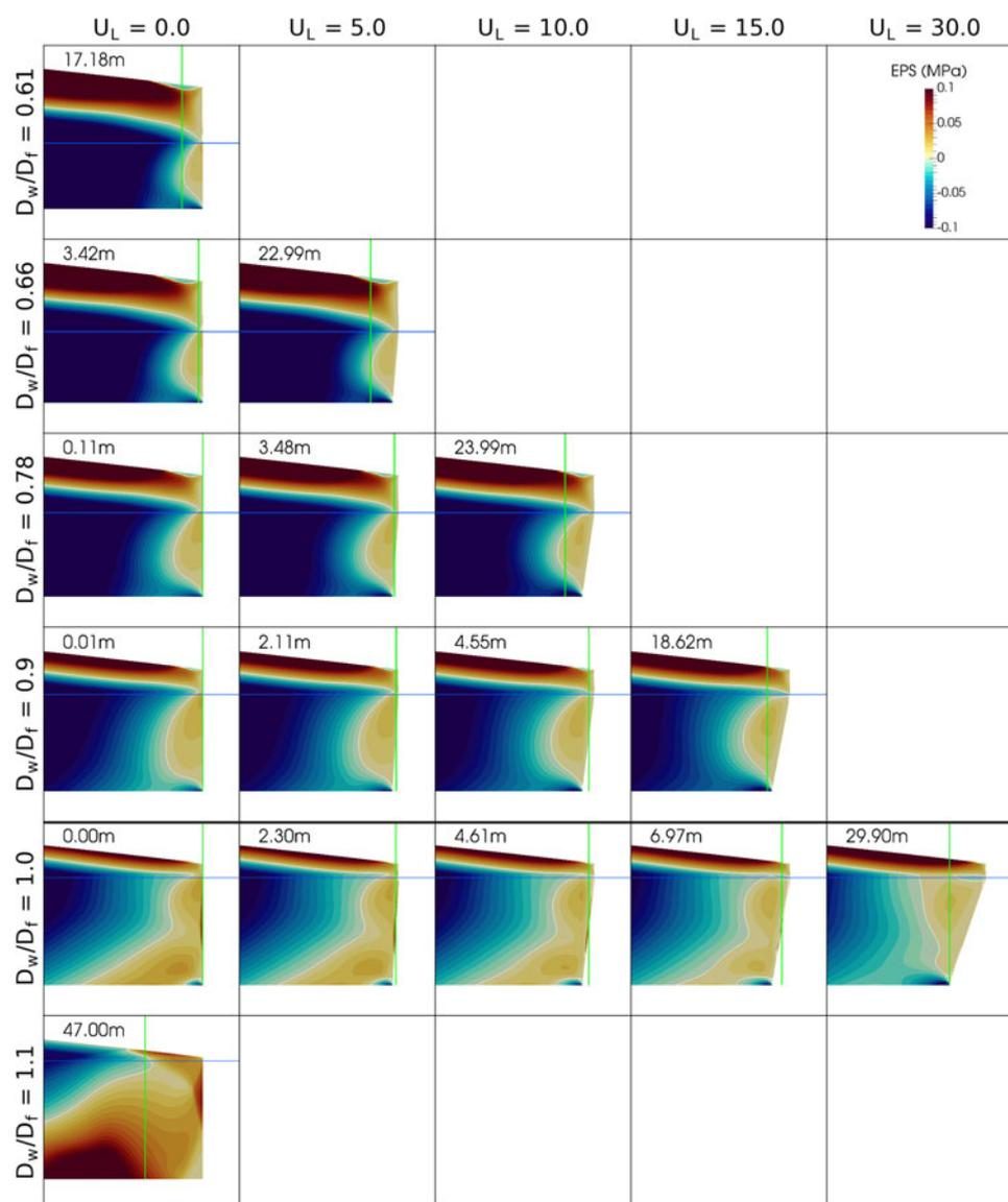
**Fig. 2.** Matrix of ice-front geometries used in the melt-under-cutting experiments, showing Effective Principal Stresses (EPS calculated in Elmer/Ice and HiDEM calving length indices (vertical green lines and figures in each panel).
