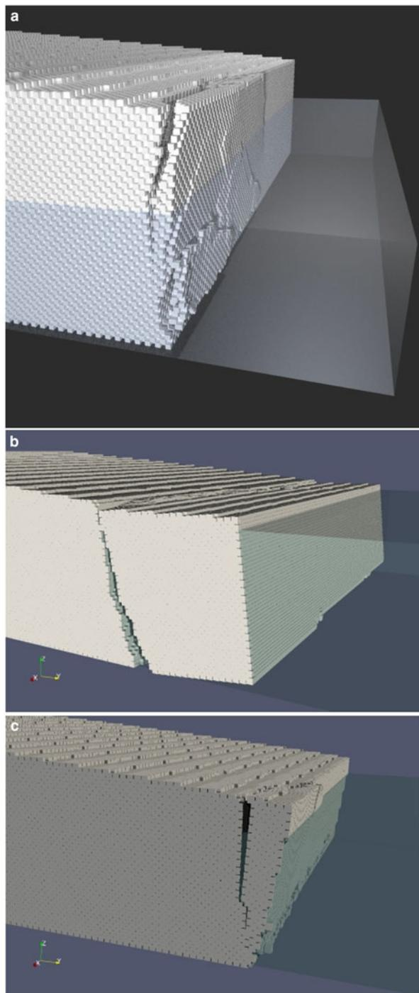
**Fig. 3.** Contrasting calving styles modelled in HiDEM. (a) Ice-cliff failure modelled using  $D_W/D_F = 0.61$  and  $U_L = 0$ . The subaerial ice face is 44 m high. (b) Buoyancy-driven calving with  $D_W/D_F = 1.1$ ,  $U_L = 0$ , showing upward growth of basal fracture and block rotation. (c) Melt-undercut calving with  $D_W/D_F = 0.9$ ,  $U_L = 20$ .
