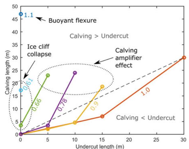
**Fig. 4.** HiDEM calving lengths as a function of undercut length for different relative buoyancies ( $D_W/D_F = 0.61, 0.66, 0.78, 0.9, 1.0$  and  $1.1$ ). The lines are intended to aid visual grouping of results, and do not imply linear variation between plotted points. Each set of connected points represents one row on Figure 2, and can be viewed as an evolutionary sequence. For each value of relative buoyancy, increasing the undercut length produces larger calving events.
