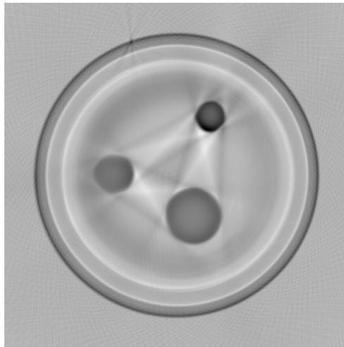
Figure 1. Example of shadow/streaking artefacts in an axial slice of a scanned laser optical CT image of a Dettol gel "finger phantom" with three strongly attenuating fingers. The region surrounding and between the fingers should be uniform grey.
