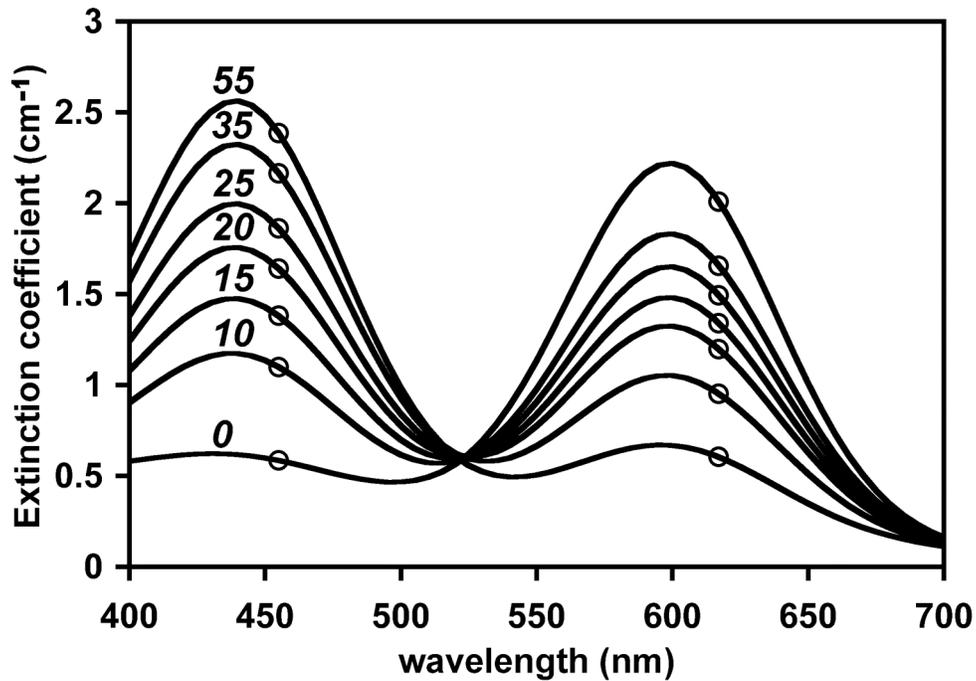
Figure 2. Modelled spectra for a hypothetical gel containing a "push-pull" pair of dosimetric pigments. Each spectrum is labelled by the hypothetical dose in gray. The open circles indicate extinction coefficients measured at two widely-spaced LED wavelengths available for use in the diffuse light source of a Vista optical cone-beam CT scanner (Modus Medical Devices<sup>TM</sup>).
