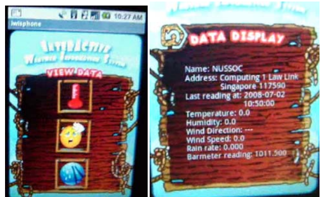
Figure 5. Left: Weather data retrieval options in IWIS prototype. Right: Weather data linkage test in IWIS (Google Android)
