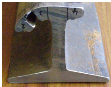
Figure 1. A cross sectional view of the rail sample
