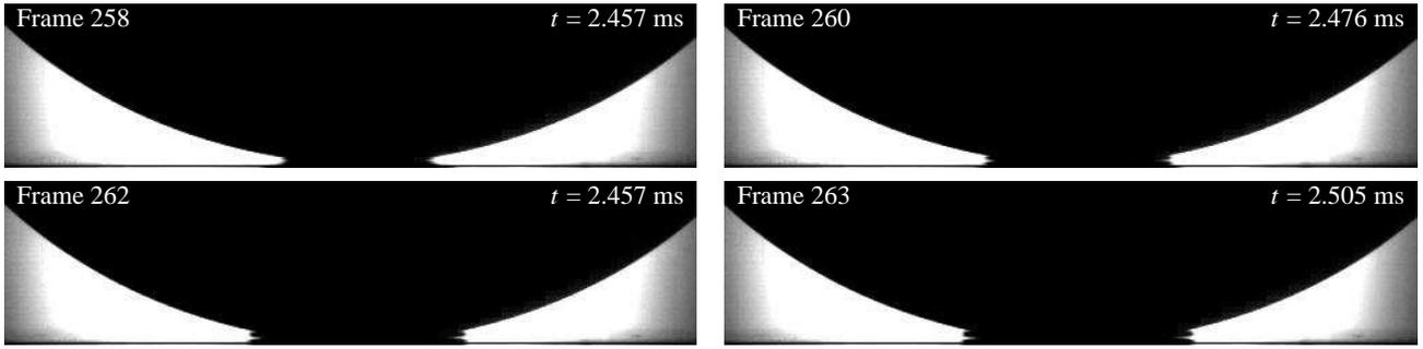
Figure 5. Images shown at frame 258 (top left), 260 (top right), 262 (bottom left) and 263 (bottom right). Frame 263 is the point of impact. The bubble is evident in the previous frames, suggesting that cavitation occurs before impact.
