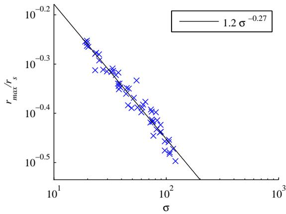
Figure 6. Maximum bubble radius vs.  $\sigma$ . Maximum bubble radius is non-dimensionalised on sphere diameter.
