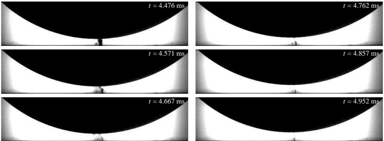
Figure 3. High-speed shadow photography images taken at 105 kHz showing cavitation bubble formed from 45 mm plastic sphere impacting stainless steel target. Every 10<sup>th</sup> image shown. The cavitation bubble pulses three times before becoming too small to resolve. The entire duration of the bubble pulses is approximately 2.2 ms.
