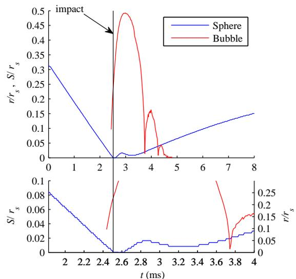
Figure 4. Sphere displacement,  $S$ , and bubble radius,  $r$ , with time. The bubble radius and sphere displacement are non-dimensionalised on the sphere radius,  $r_s$ . The first instance of the bubble occurs in frames preceding the minimum displacement of the sphere, suggesting that cavitation may occur before impact. Detailed view in bottom plot, where sphere displacement is not smoothed.
