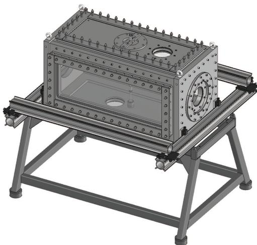
Figure 1. The variable-pressure Bubble Dynamics Chamber has a test volume of 520×520×1200 mm. The short ends and two opposite long sides (top and bottom) are stainless steel plate. The remaining sides are 85 mm thick acrylic windows. The chamber can be operated at pressures from 10 to 400 kPa.
