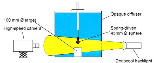
Figure 2. Schematic of the experimental setup showing location of sphere, target, high-speed camera, diffuser and backlight. The compression spring to accelerate sphere is housed within the sphere-tube assembly and not shown.
