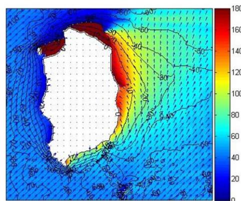
Figure 8. Changes in wave direction during the south westerly wave
