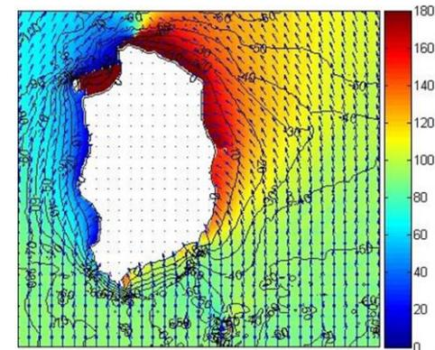
Figure 9. Changes in wave direction during the southerly wave
