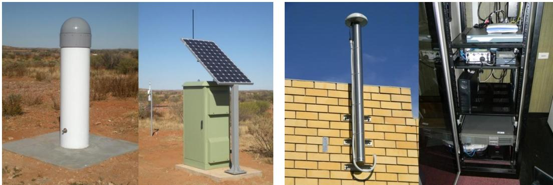
Figure 2: Typical CORSnet-NSW monumentation and auxiliaries at Tier 2 (left) and Tier 3 (right) sites
