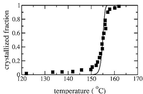
FIG. 3. Crystallized fraction of the GST material as a function of temperature during a ramped anneal with a heating rate  $3$  °C/min starting at  $120$  °C. The line shows the result of simulation using our model, while the squares are experimental data from Ref. [35].
