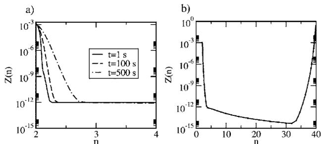
FIG. 2. Numerical solutions of the master equation (1). (a) Initial iterations for  $T=140$  °C. (b) Final cluster size distribution profile for  $T=140$  °C—the final profile is determined by the exhaustion of monomer.
