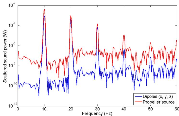
Fig. 3: Comparison of the radiated sound power produced by the dipoles and the FW-H generated incident pressure field
