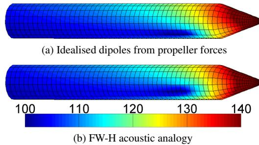
Fig. 2: Incident pressure on the submerged shell. Pressures in dB (ref.  $1 \times 10^{-6}$  Pa)
