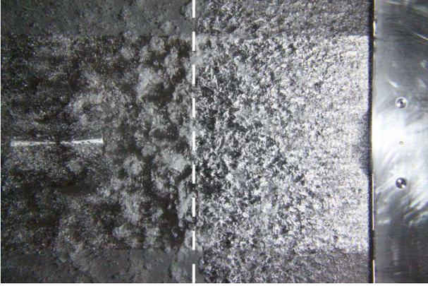
Figure 3. Image of a ventilated cavity detaching from a BFS for  $\delta/h = 2.0$  &  $C_{Qv} = 0.027$ . The 2-D nature of the cavity is apparent indicating that the ventilation flow is sufficiently distributed across the span of the step. The cavity closure is identifiable (indicated by the white dashed line) with air discharging from the closure region in shed cloud cavities and individual bubbles. Flow is from right to left.
