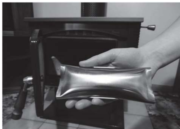
Fig 2. Catalytic combustor (15cm long) used in this program.
